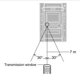
Aim at the sensor, avoiding obstacles, at a maximum range of 7 meters directly in front of the unit.
